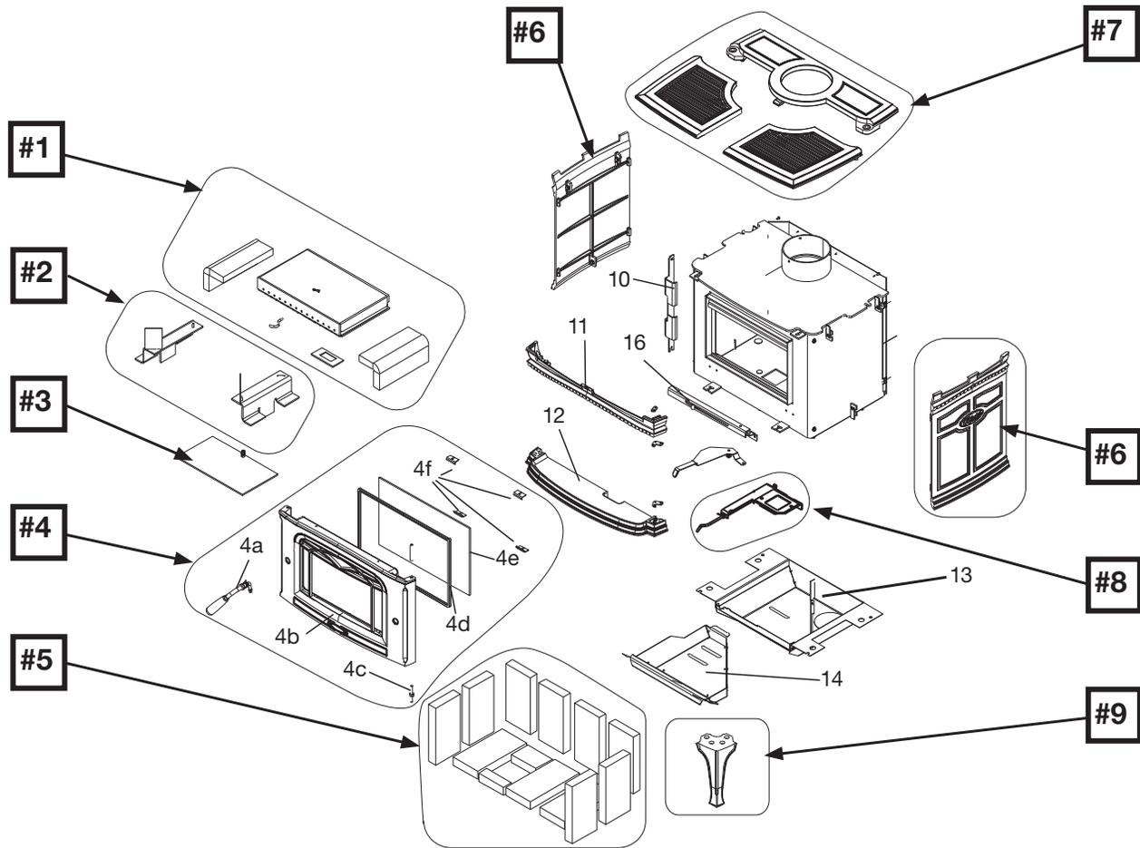
Figure 8. ALT4 AS Replacement parts.
